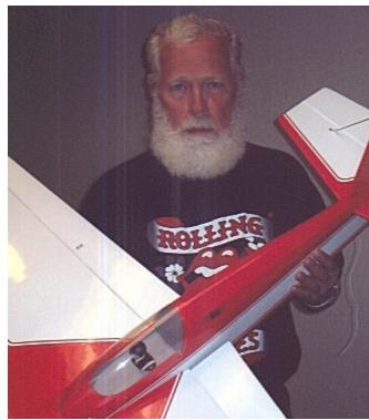
Above: Kent Struwe with his "Somethin' EXTRA" ARF by venerable Sig Mfg. of Montezuma, Iowa, with a 51 inch fully symmetrical wing span, 670 sq.in. of area, and weighing just under 6 lbs., including its OS.50SX engine.
