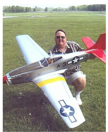
Above: Jim Strelitzer, with his P-51 Mustang giant scale, 84 inch wing span, 23 lbs., 1,245 sq. in. wing area, powered by a Desert Air DA-50. Done in WW II Tuskegee Airman colors: red spinner & tail feathers. Jim's pilot even has brown skin, and Jim has conversed with the WW-II pilot (2<sup>nd</sup> Lt. George E. Hardy), now retired in Florida.
