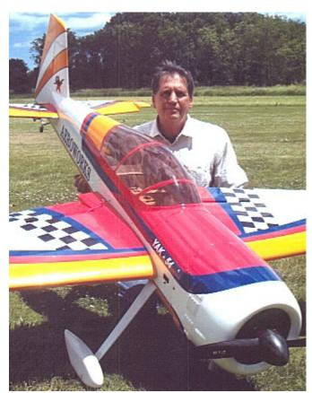
Don Finney at the field with his new 35% Yak,104 inch span, weighing 27.5 lbs., powered by a Desert Aircraft 6.0 cu.in. twin cylinder engine, 27"/10" prop.
