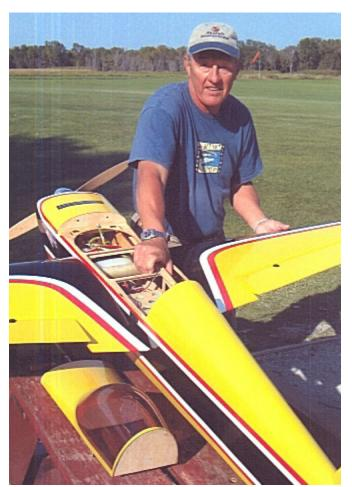
Above and lower left: Dennis Bartz assembling his ARF "Edge" of some 92 inches wing span, 22 lbs weight, powered by a Lanier .75cc 3W engine.
