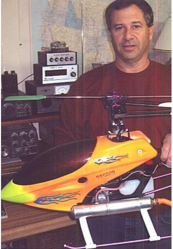
Above: Chuck Bucci holding his .50 cu. in. engine radio controlled Raptor helicopter, - 26 inch blades.
