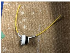
From the workbench of **Angie Traut**, Angie figured out that if you don't have a pair of tubing benders, you can string a piece of 3D printer filament through the tube and bend it by hand without fear of the tube kinking up or breaking. In this case, the Ninjaflex 1.75mm fits through the standard 1/8" brass tubing that is supplied with most fuel tanks. This would also work well in conjunction with the bending tool.
