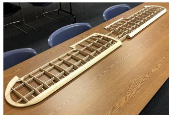
Todd Schmitt started working on a Sig J3 Cub kit and brought in its wing. It will have a 74" wing span covered in monokote and Todd is still considering its power source.
