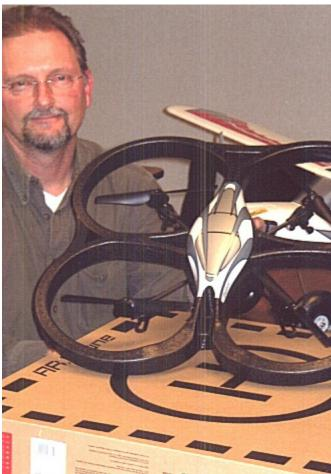
Above: Marty Gscheidmeier flew in the room his new electric power "AR Drone Quadracopter" purchased for \$299 at the Brookstone store in Mayfair. It is controllable by the Apple ipad or similar devices. Hovers or tilts to aim on-board camera. Stabilized by ultrasonic sensors and accelerometers.
