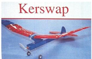
Above: The Kerswap model Brad DeLellis is currently building from a 1940's design by Gilbert Morris when Morris was age 18. It will have 400 sq. in. of wing area, a 52 inch span, and weigh up to 4 lbs. with the electric motor and its battery. Morris came up with the "Kerswap" name from the sound of a model landing hard. Morris is still alive, at age 88.
