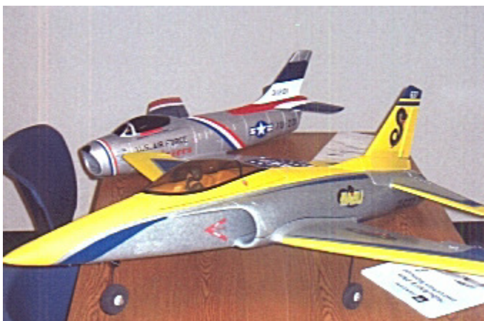
Above: Tom Ryan's pair of foam electric internal ducted fan propulsion. The F-86 was shown last month unassembled. It tears off its wing fuel tanks intended for belly landing. Tom will try a sturdier mount for them. In flight it is very fast. The HABA BNF Viper gears actually work, rare for a foamy.
