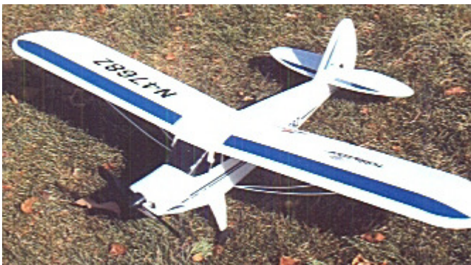
Above: John's Cessna-like trainer, all foam electric motor from "hobbyzone", with Spektrum radio.
