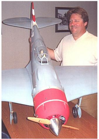
Above: Duane Gagnon with a rare Lavochkin LA-7 Russian WWII fighter. It looks like a cross between a German FW190, and a USA P-47 Thunderbolt. The 17 lb. ARF is from Top Flight Models of Chicago, has an 80 inch wing span, powered by a 1.80 Saito 4-cycle. Below: Front view of mock radial engine insert.
