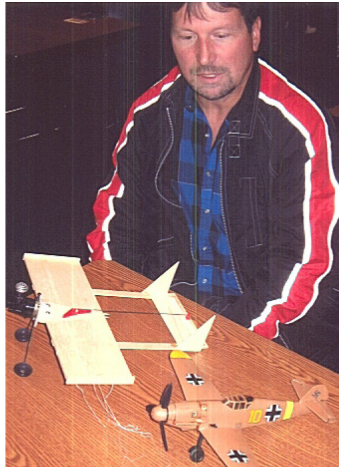
Above: Steve Ward showing revivals of some of his .049 control line models. The balsa version has a Cox engine with attached fuel tank & needle valve assembly; the plastic Messerschmitt has an integrated .049 of uncertain make, 1970s vintage.
