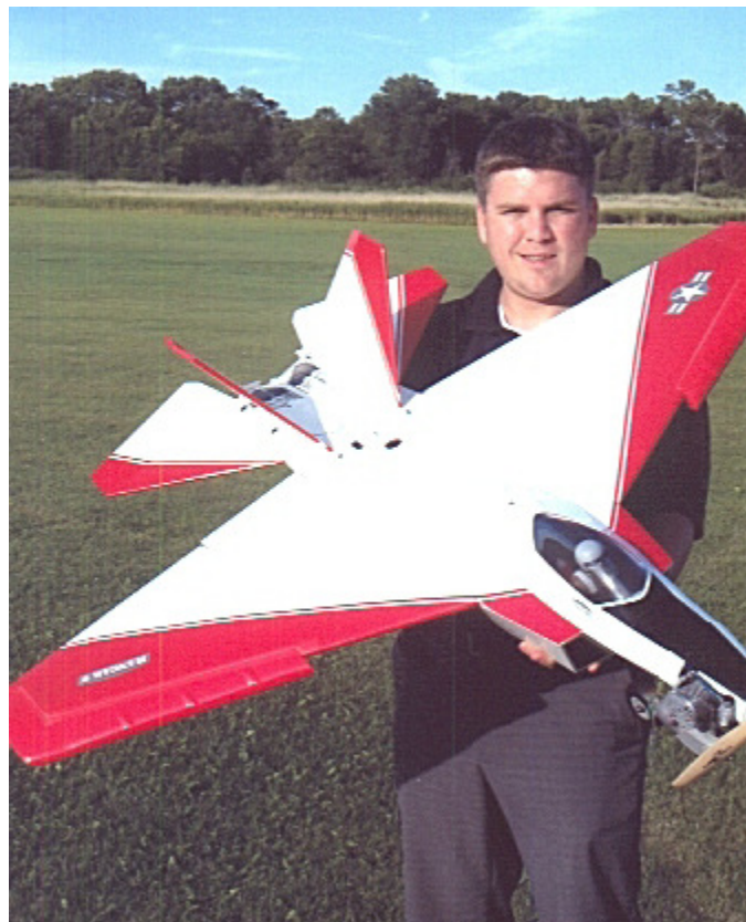
Above: Joshua K. Alwine at the field with his F-22 Raptor by Hanger 9, powered with a .46 Evolution engine. Flaps are necessary to lift the 8 lbs. during takeoff. Under-cambered outer wing panel “droops” and tip winglets help avoid liftoff and landing stalls.
