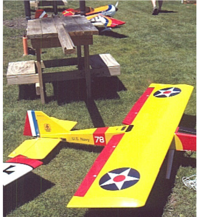
Above: Foreground: Del Fisher's electric Eflite ARF, 76" span 9 cell E110 motor, in "between the wars" color scheme; mid-picture one of Bob Kabella's wing restraint type pit tables; background, Jim Strelitzer's DA 50 powered (with smoke system), 86 inch span.
