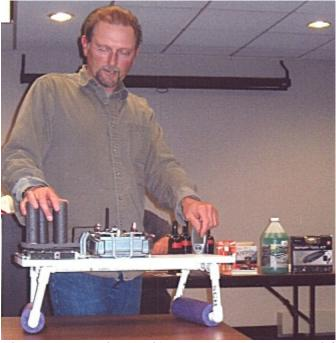
Above: Marty explaining his Transmitter tray system, left hand on flight timer, right hand on sliding tray gripper pegs.
