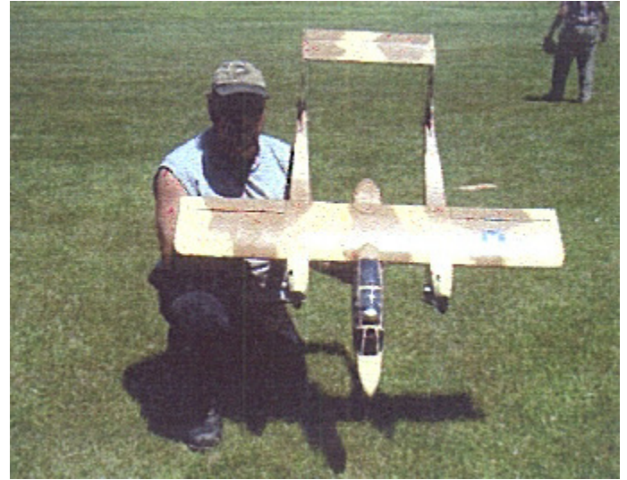
Above: Hidden in the shade of his hat is Rich Kegel showing a Bronco OV10 ARF by Netco Models with 48" wing span, twin OS .15 engines, controlled by 9 servos, colored by Testor's model paint, fuel proofed with clear overcoat..
