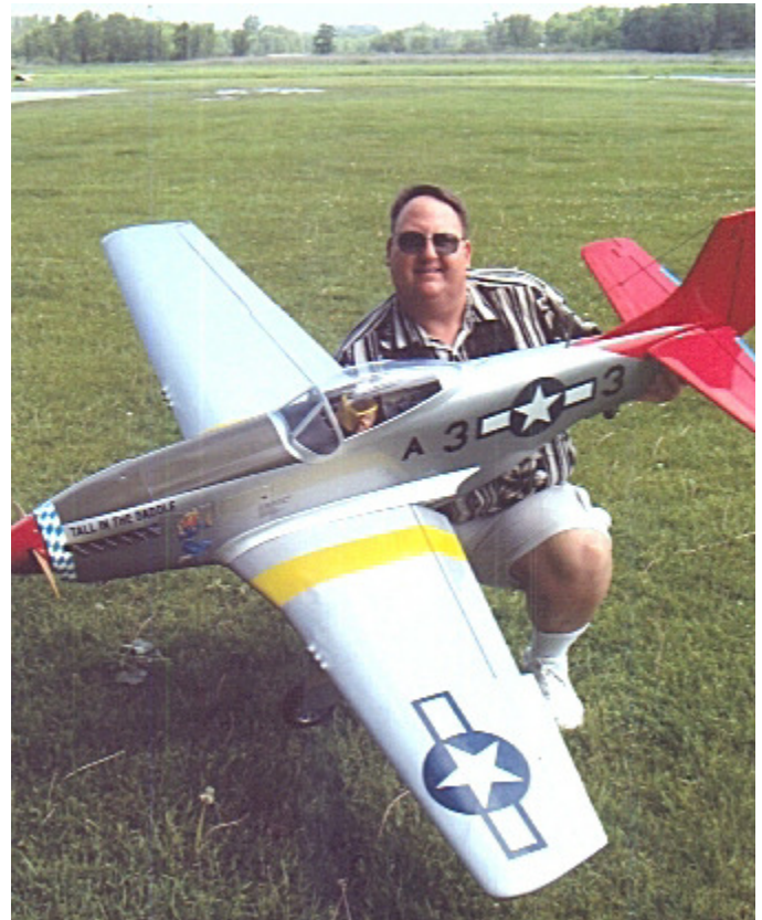
Above: Jim Strelitzer, with his P-51 Mustang giant scale, 84 inch wing span, 23 lbs., 1,245 sq. in. wing area, powered by a Desert Air DA-50. Done in WW II Tuskegee Airman colors: red spinner & tail feathers. Jim's pilot even has brown skin, and Jim has conversed with the WW-II pilot (2 nd Lt. George E. Hardy), now retired in Florida.
