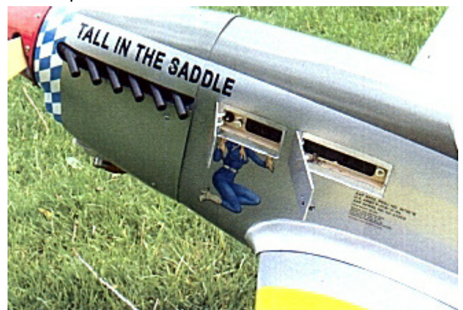
Above: Close-up photo of access doors to fueler, air supply for pneumatic retracts, and on-off switches. Engine exhaust stacks are operational via custom exhaust by Keleo Creations. Graphics by Cal-Grafx.
