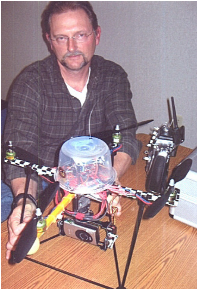
Above: Marty Scheidmeier displayed and explained his European kit-made electric powered “flying platform,” with pendulum suspended camera.
