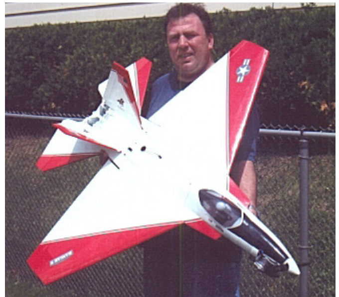
Above: Bob Ehlers with his Hangar 9 F22 Raptor, .45 cu in Evolution engine, 48" span, 675 sq in, 7-1/2 lbs. Canopy lettering dedicated to his father, William Ehlers, F-86 pilot.
