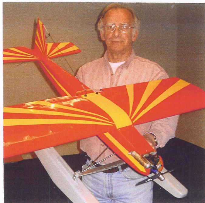
Marv Bishop with his Floyd Katz designed and built trainer, this one on floats, .15 cu.in. engine.
