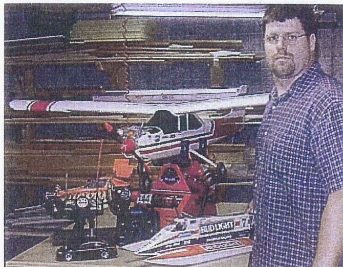
Craig Manka with his Hobbico "Nexstar Trainer", OS .46 ABC engine, 69 in. wing span, 722 sq.in. area, 6.5 lbs. and other R/C equipment - car, off-track, and speed boat.
