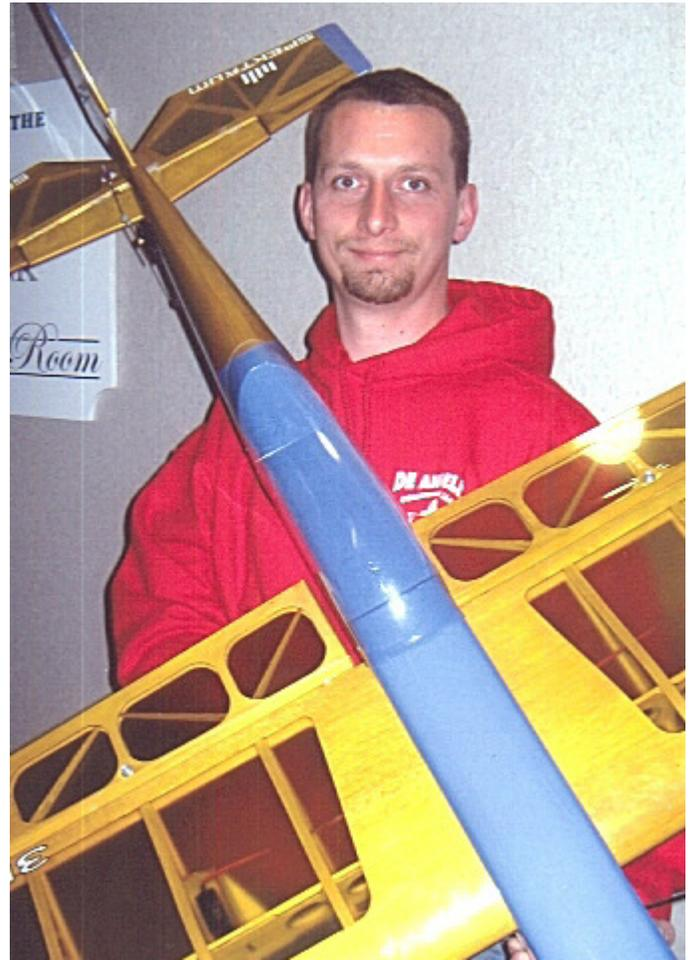
**Above:** Shawn Rehm displaying his 3D Passion ARF from Nitro Planes at the March, 2009 club meeting. It has an OS.61 engine to power the 6.6 lbs. of weight, being lifted by a 55 inch span wing, and controlled by ailerons that are 3 inches wide at the wing tips and 4 inches at the wing root. "3D" means capable of vertical attitude flight, hanging motionless.
