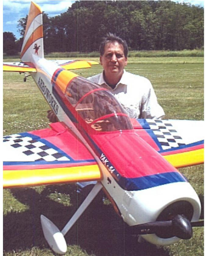
**Don Finney at the field with his new 35% Yak, 104 inch span, weighing 27.5 lbs., powered by a Desert Aircraft 6.0 cu.in. twin cylinder engine, 27"/10" prop.**
