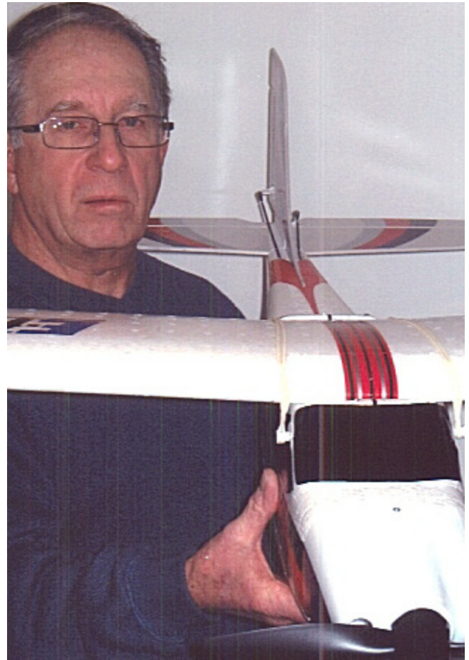
Above: Charles and his electric motor "Apprentice" by E-Flite, a 3 lb., all-foam, 55 inch wing span trainer.
