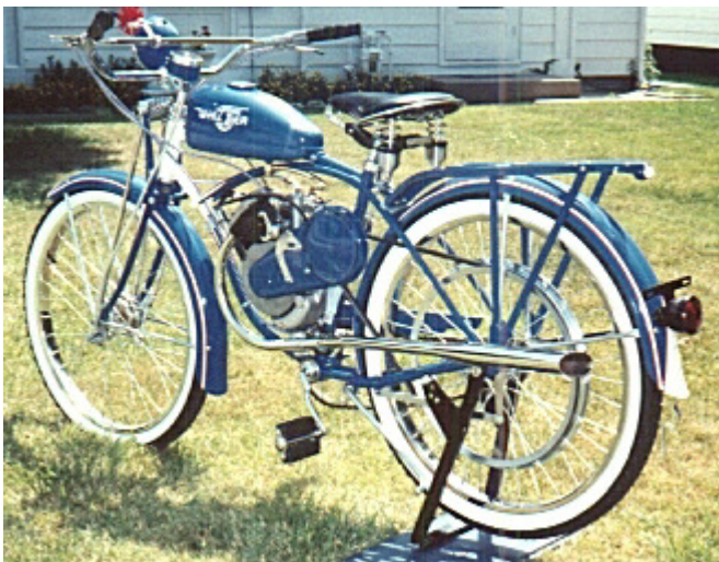
Above: A 1951 Whizzer 3 hsp motor bicycle made in Pontiac, MI. Restored "ground-up" (early 1980s) by Charles Christoffersen, including detailed paint job.
