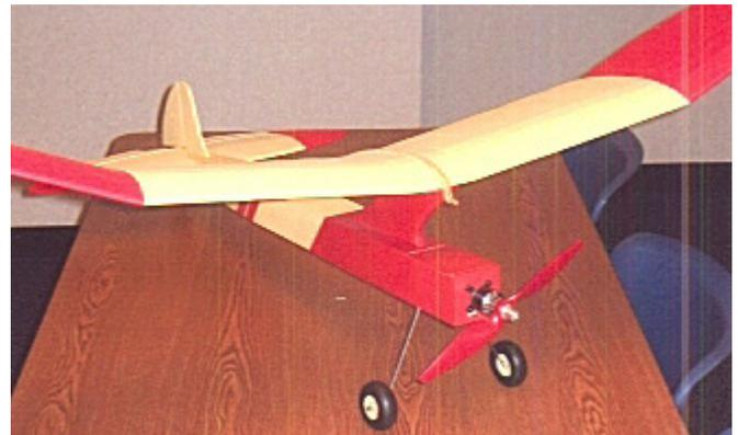
**Above:** Close up of DeLellis model finished with fabric-like Solar Tex covering.
