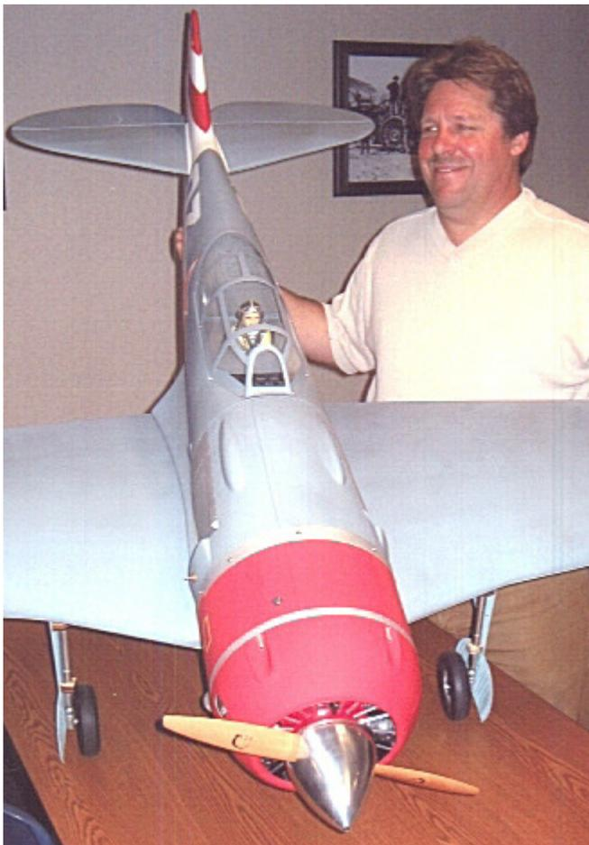
**Above:** Duane Gagnon with a rare Lavochkin LA-7 Russian WWII fighter. It looks like a cross between a German FW190, and a USA P-47 Thunderbolt. The 17 lb. ARF is from Top Flight Models of Chicago, has an 80 inch wing span, powered by a 1.80 Saito 4-cycle.
