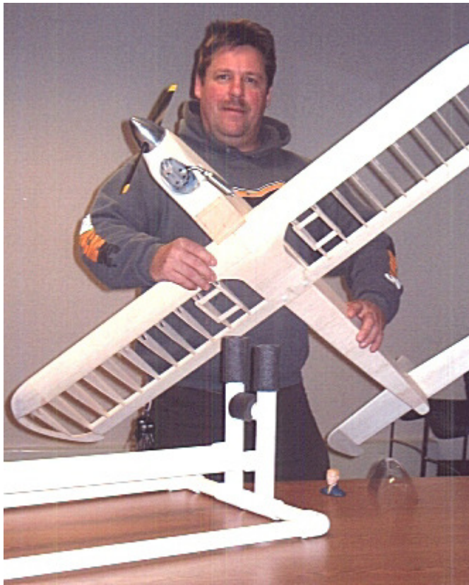
Above: Duane Gagnon and his 1970's "Smoothie" kit by Balsa USA ($70) that he is now building. This bottom view shows the inverted .52 cu. in. Magnum 4 stroke engine neatly cowled in, and the "smooth lines" of the wings. The plans call for a 2 stroke .35-40 cu.in engine.
