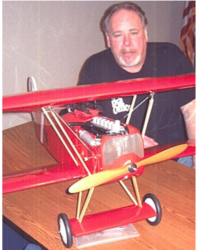
Above: Rich Kegel and his completed Sterling kit of a Fokker DVII shown uncovered at the January, 2010 meeting. The kit is 30 years old, had many small parts and plastic parts had gone brittle. The Saito. 62 4-cycle engine is now nicely obscured by the cowling mesh. Wing area is 950 sq. in., with 1.5 lbs. lead in the nose to balance. The Williams Bros. machine guns require assembly of 30 individual parts!
