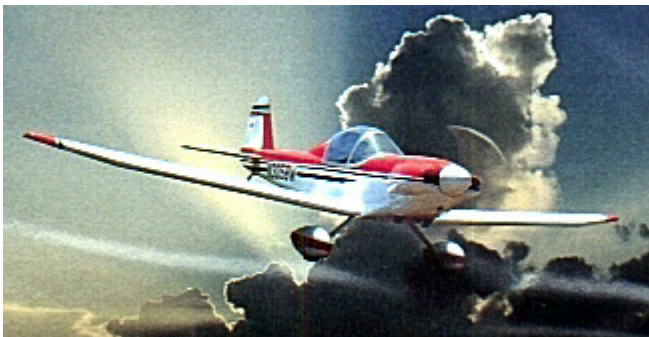
Above: Artist's rendering of the Thatcher "cx4 Sport Aircraft" being homebuilt by Ken Ceranski. It will be 18 ft. long, 24 ft. wingspan, weigh 850 lbs;125 mph cruise, 65 hsp. hor.4 cyl. Volkswagen engine.
