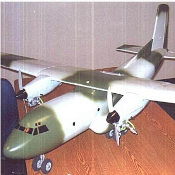
Above: Duane Gagnon and his C-160 cargo lifter same as Darrell Hossalla showed last month, but in original camouflage colors, not U.S. Coast Guard white as repainted by Hoss. Engines: Twin .30 Magnum 4 cycle, inverted. Below: 3/4ths view.
