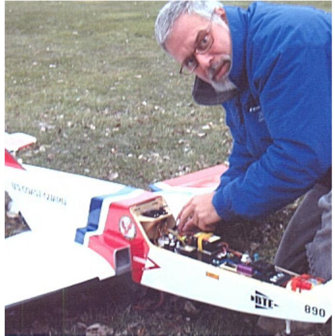
**Jeff Borowski and his all-balsa wood, Reaction 54 jet model, 78 in. wing span, 1,453 sq.in. wing area, 18 lbs. weight and 18 lbs. of engine thrust. The wing has a 24 inch chord and is 4 inches thick, which make for great controllability at all speeds, including hovering on mild headwinds, rare for jets.**
