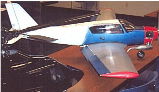
**Above: Duane Gagnon's Piper Comanche (prototypes had P-51 Mustang wings,) Jack Stafford 1995 kit, with retractable landing gear, flaps,.75 Supertigre engine, Darrell Hossalla helicopter in foreground.**
