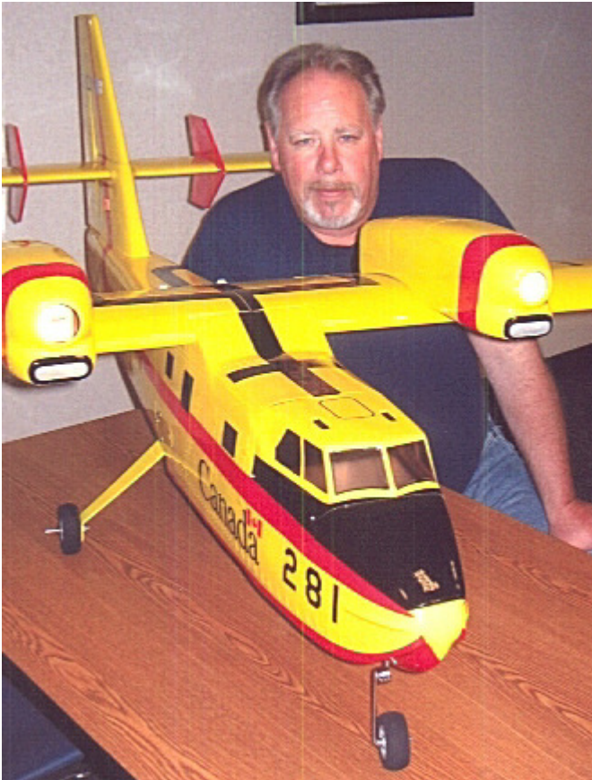
Above: Rich Kegel and his CanadaAir CL 415 land & sea water bomber for fighting forest fires. The prototype contains a bottom water intake scoop to refill its tanks by skimming a lake or river, allowing it to quickly return to the fire area. It is a turbo prop (2300 hsp each side of the original). The model: .72 Saito 4cycle inverted engines, on-board glow igniters.
