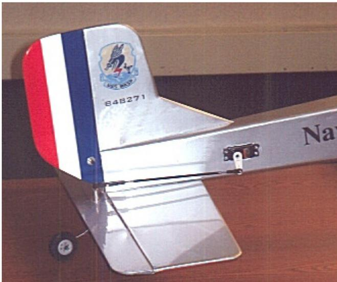
***Above: Tail view showing example of kit modifications, where vertical fin is squared off, and elevator servo is rear-mounted, with exterior clevis system.***
