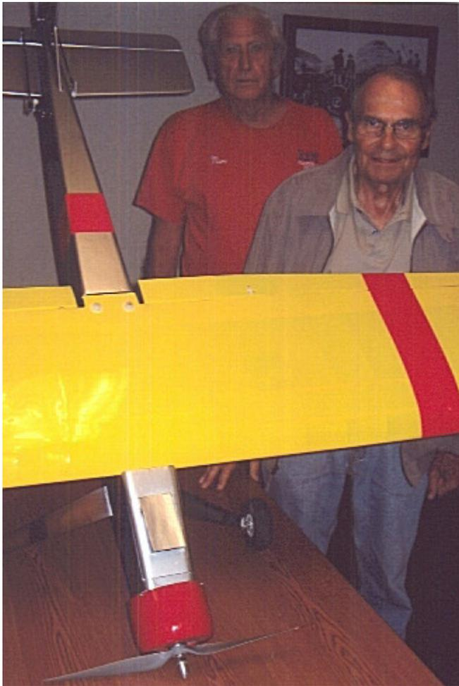
***Above: (Rear) Marv Anderson, builder, and (front) Dell Fisher, owner, of a large Mystery Stik, 67" span, set up for an electric motor (Hacker brushless, 1300 watts). Many kit modifications, including cowling.***
