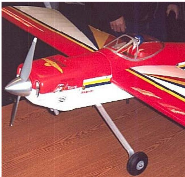
Above: Bill Flannery's Lanier 60 ARF with a Super Tigre .90 engine, 60 inch wingspan, and after-market fibreglass cowl to replace the weaker version of the ARF kit. The model assembled had tail weight issues, which Bill corrected.
